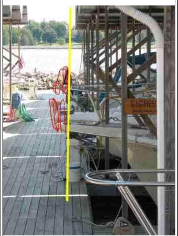
This picture represents the manor in which the vessel over hang is measured for a Bow Pulpits Over Hang ** NOT In Compliance **
