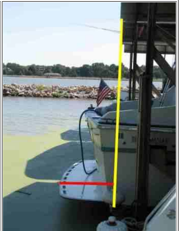
This picture represents the manor in which the vessel over hang is measured for a Stern In Bow Over Hang.
