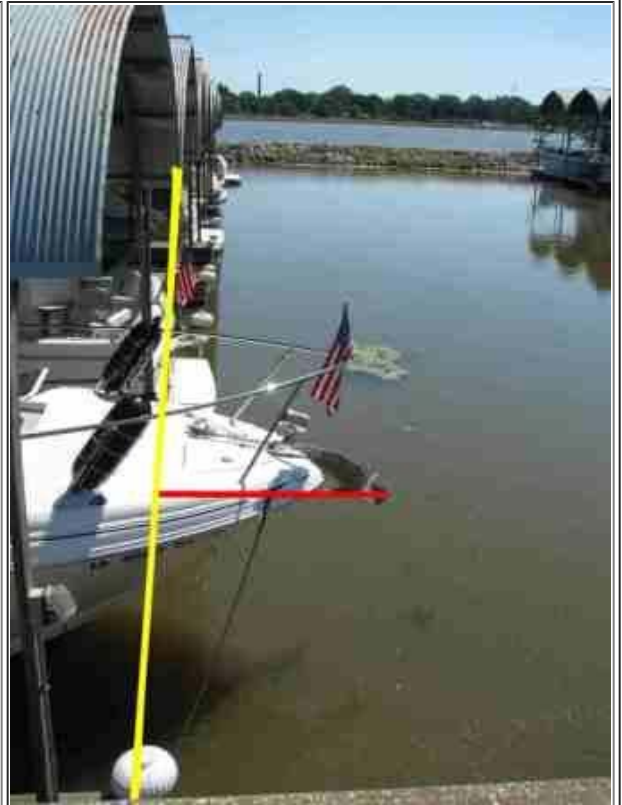
This picture represents the manor in which the vessel over hang is measured for a Stern In Bow Over Hang.
