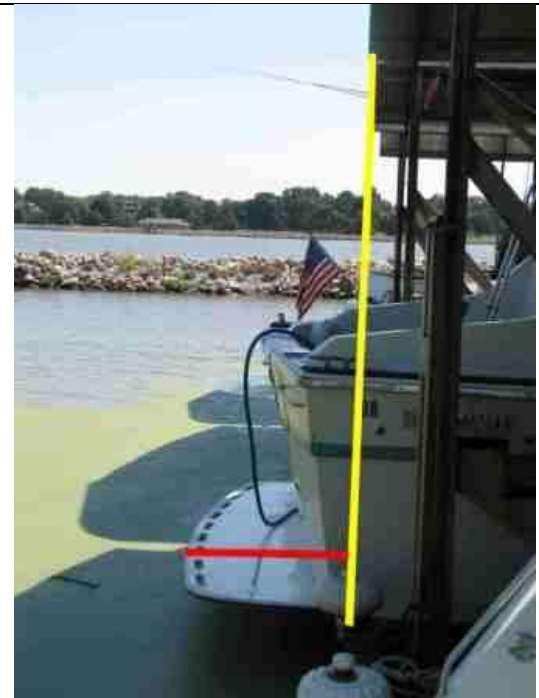
This picture represents the manor in which the vessel over hang is measured for a Swim Platform Over Hang.
