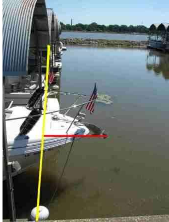
This picture represents the manor in which the vessel over hang is measured for a Stern In Bow Over Hang.
