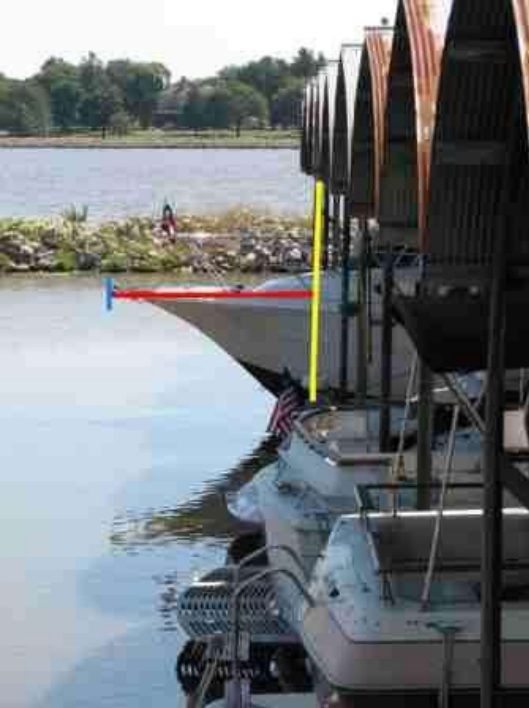
This picture represents the manor in which the vessel over hang is measured for a Stern In Bow Over Hang.
