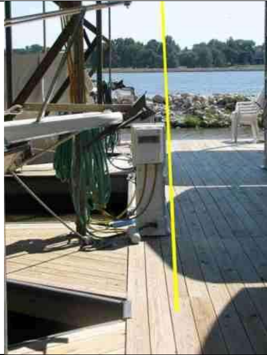
This picture represents the manner in which the vessel over hang is measured for a Bow & Stanchion Over Hang ** In Compliance **
