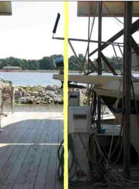
This picture represents the manner in which the vessel over hang is measured for a Bow & Stanchion Over Hang ** NOT In Compliance **
