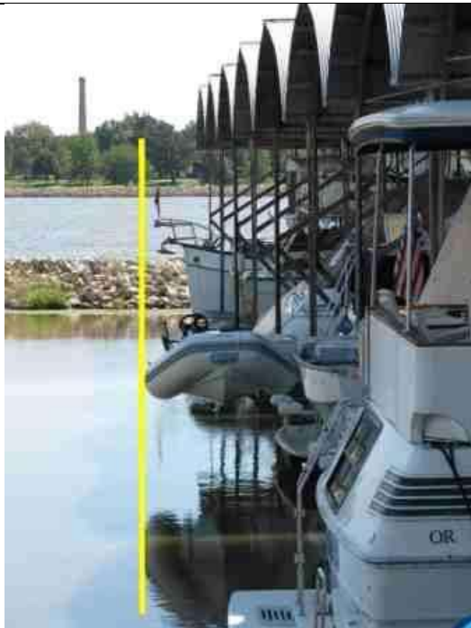
This picture represents the manor in which the vessel over hang is measured for a Attachments Over Hang.
